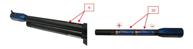
Unscrew the screws emitters / 9 / and you pull the emitter. Inside is space for two 1.5V AAA batteries / 10 /. The batteries insert into the emitter. Put the emitter on the work arbor and screw the screws / 9 /. When inserting the batteries, you must observe polarity.
