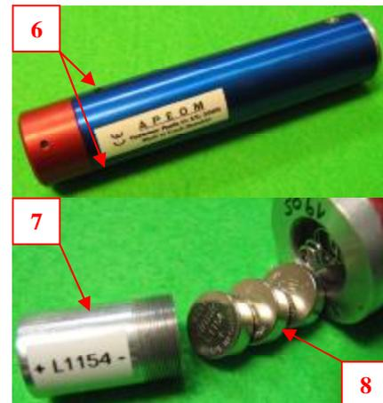
Do not short-circuit the batteries, do not dispose of them in a fire. Do not combine batteries made by various manufacturers or of various ages in one emitter.
